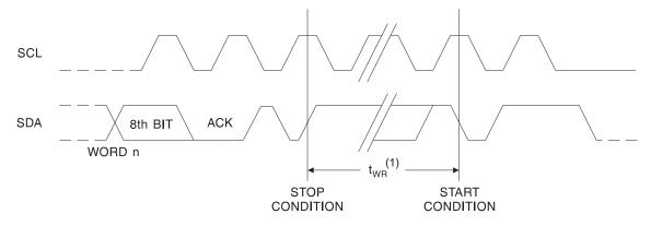
The write cycle time t<sub>WR</sub> is the time from a valid stop condition of a write sequence to the end of the internal clear/write Note: cycle.
