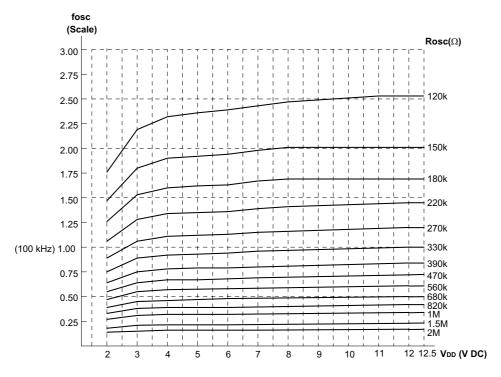
The recommended oscillator frequency is  $f_{OSCD}\left(decoder\right)\cong f_{OSCE}\left(encoder\right)$
