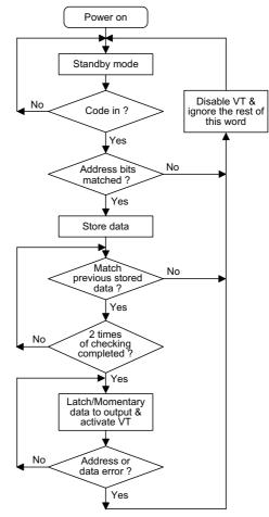
Note: The oscillator is disabled in the standby state and activated as long as a logic "high" signal is applied to the DIN pin. i.e., the DIN should be kept "low" if there is no signal input.
